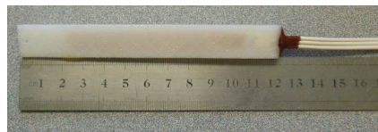
Figure 3.1. Embedded strain gauge for monitoring shrinkage deformation
