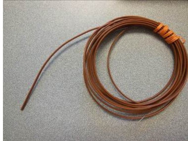
Figure 3.2. Thermocouple used for concrete temperature measurement
